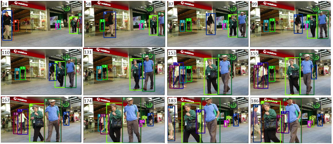
Figure 1.1: In the above diagram the numbers on the top left represent the frame number with detection bounding boxes in red and track bounding boxes in other colors. The above diagram depicts the occlusion handling done by our system. It can be seen that track 5 (blue) observed in frame 24 is well tracked through out even after been occluded, given that the maximum occlusion duration is less than 30 frames. Additionally tracks 17 and 19 (blue and purple) are reidentified in frame 183 after been occluded. This is because, we control how much the occluding image’s features can affect the track’s template when the track is partially occluded
